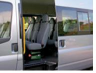
seats are fitted with lap-and-diagonal belts and adjustable headrests and the 12-15- and 17-seaters come with a Schedule 6 pack.
